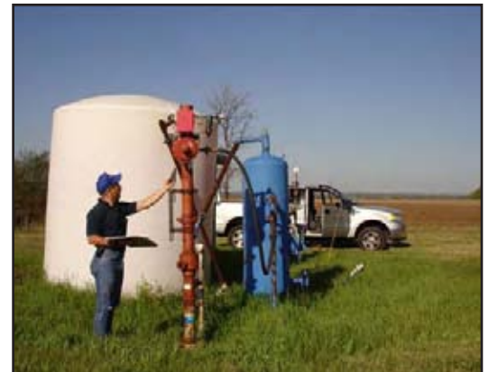
DEC staff person inspects a producing gas well. A new rust-proof tank helps prevent leaks at the site.
