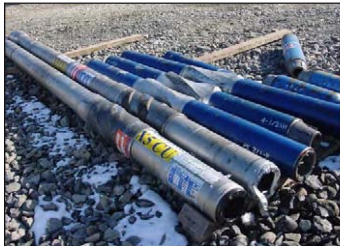
Schlumberger directional drilling assembly photographed at Fortuna Energy's Drumm #1 well in Steuben County. A directional drilling assembly allows the driller to control the direction of the wellbore while a well is being drilled. This type of tool is used to drill horizontal or directional wells.
