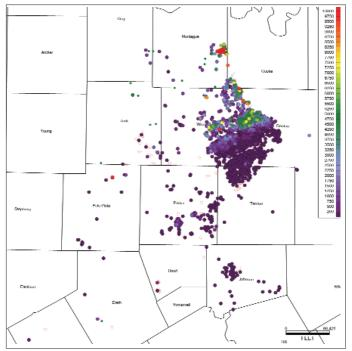
*Figure 2.* Normalized six-month cumulative oil production shows low oil output in the core sweet spots for gas.
