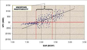
Figure 4. Cross-plot of full project net present value versus average estimated ultimate recovery per well with pilot and mid-program thresholds.
