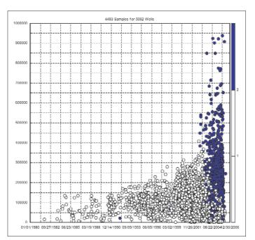
*Figure 4.* In this production timeline, the blue dots are horizontal wells, a game-changer that greatly increased Barnett gas production.
