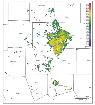
**Figure 1.** The best Barnett Shale vertical gas wells are shown in orange or red, the lowest producers are in purple.
